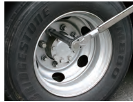
Extra long Socket for wheel nut
